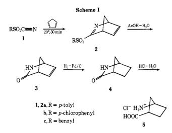
The spectral data of 2-5 (see Experimental Section) agree with the proposed structures. However, for 4 there is a conflict with literature data. Recently, the groups of Moriconi<sup>8</sup> and Paquette<sup>9a</sup> independently assigned structure 4 to a product obtained through the addition of chlorosulfonyl isocyanate (CSI) to bicyclo[2.1.0]pentane (7, Scheme II). Their spectral data do not agree with those
